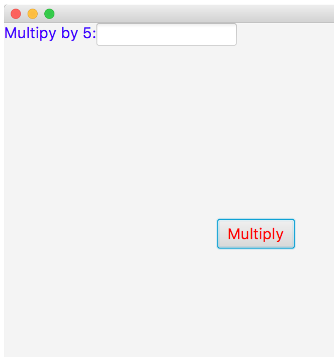
Figure 1.14: What our GUI looks like with Java running it with a width of 400 pixels and a height of 400 pixels.
