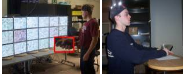
Figure 12. a) Image showing a participant using the gyro mouse with the display. The gyro mouse is enlarged in the red square. b) An image showing the hat used to track users' position.
