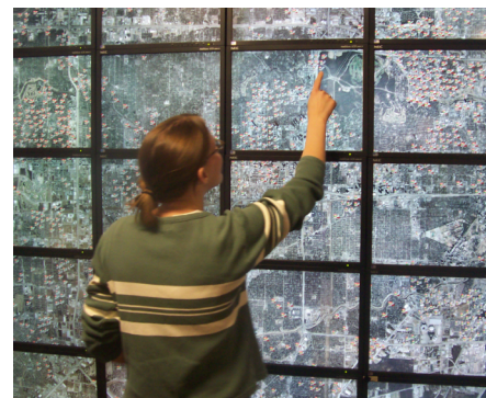
Figure 1. 100 MP 50-monitor display condition that allows both physical navigation and peripheral vision. The total resolution of the display is 16000 X 6000 (96,000,000 pixels).
