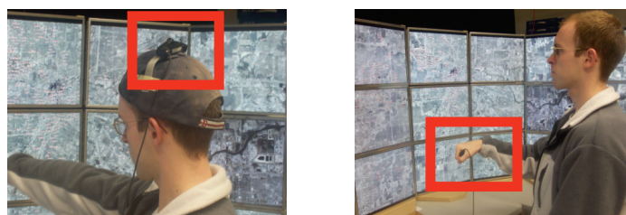
FIGURE 4: a) A participant using a head tilt tracker, highlighted by the red rectangle. b) A participant using a hand-head tilt tracker, highlighted by the red rectangle.
