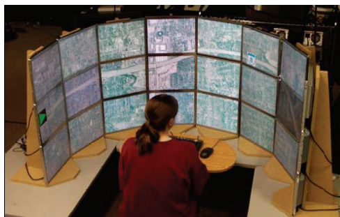
FIGURE 2: A user in the middle of a curved desktop display. If the monitors used are touch screens then the user can use less effort to touch any screen than if the display were flat.
