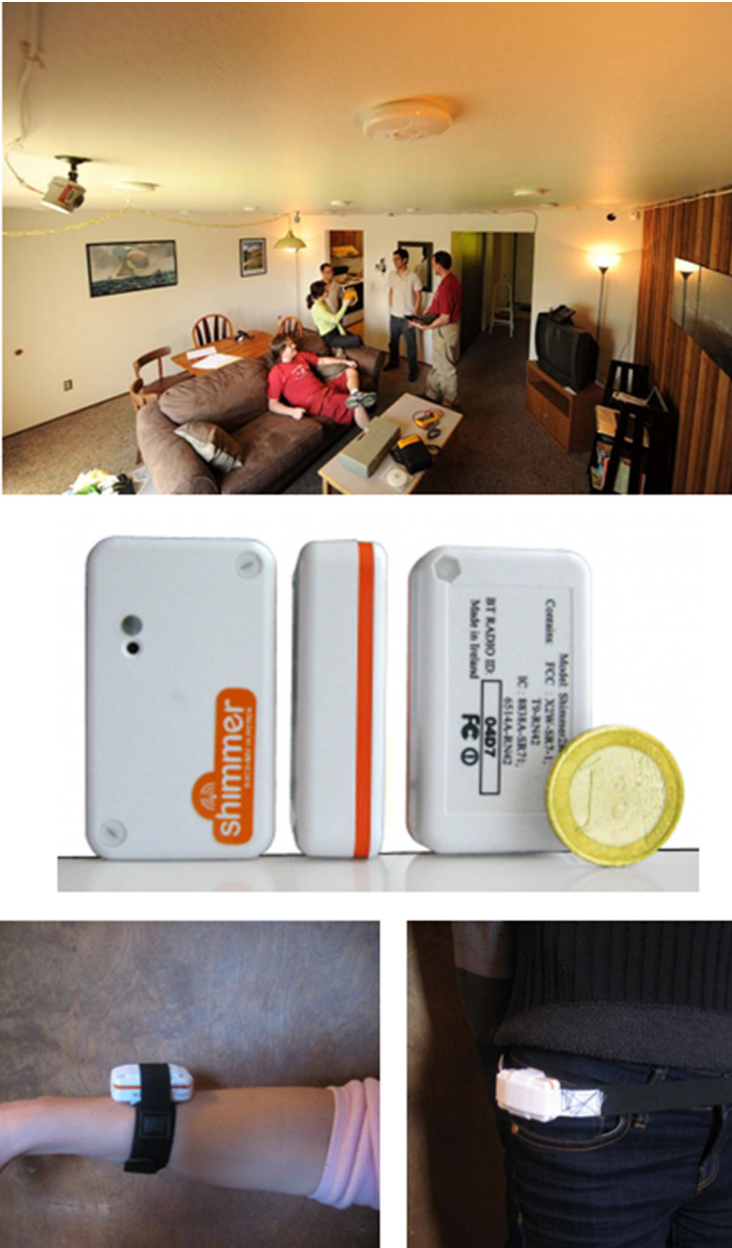
Fig. 6 Motion ( top ), object ( middle ), and accelerometer ( bottom ) sensors in the home
